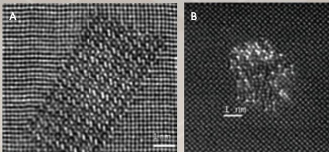
**A.** Ordered precipitate without Cu. **B.** Disordered precipitate with Cu. In both images, the aluminium host lattice can be seen around the precipitate. HAADF-STEM images taken by Sigurd Wenner, Takeshi Sato and Calin Marioara.
