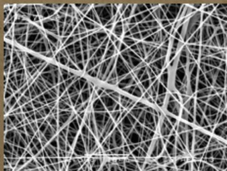
A scanning electron microscope (SEM) image of an electrospun nanofibre mat.
