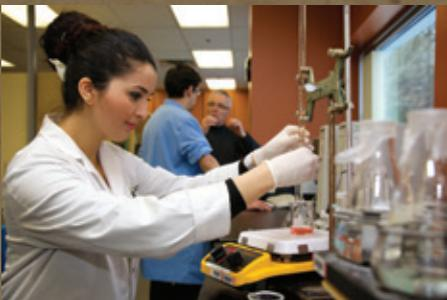
A PhD student determining copper ion concentration in effluent via titration after adsorption test with nanofibres.
