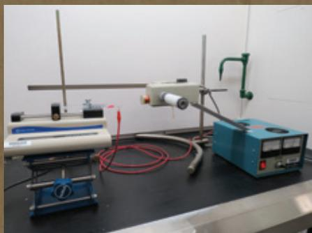
Apparatus used to make nanofibres by electrospinning.
