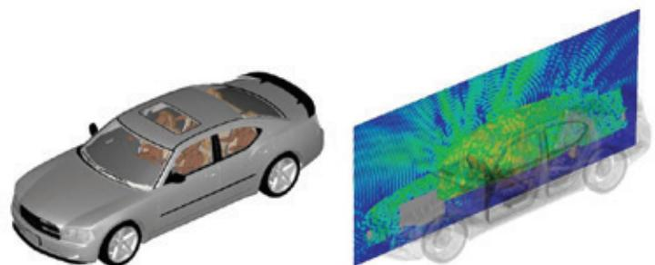
Car model with mobile device radiating at 2 GHz simulated with 1.5 billion FDTD grid cells.
