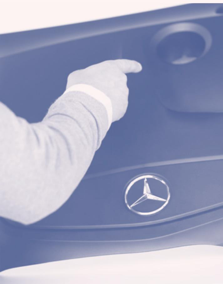
Mercedes Benz A-Class engine cover made from 70 per cent bio-based EcoPaXX.
